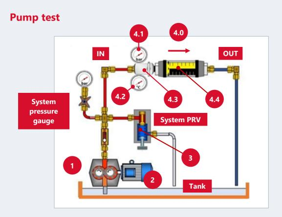
Figure 8: Schematic diagram of pump test
