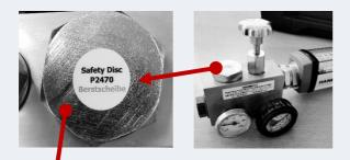
Figure 11: Power meter with burst pressure protection
