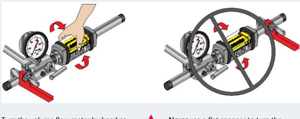
Turn the volume flow meter by hand so that you can see the display scale.
