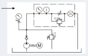
Figure 9: Hydraulic diagram of pump test
