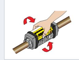
Turn the volume flow meter by hand so that you can see the flow scale.
