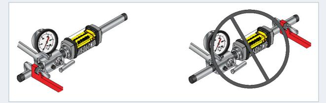
Attach the wrench on the same side on the valve body on which the pipeline is tightened.
