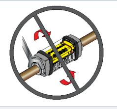
**Never** use a flat spanner to turn the protective casing in order to view the flow scale.
