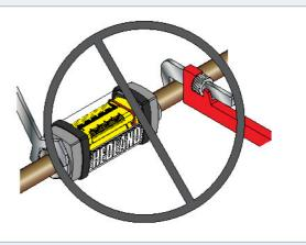
Attach the flat spanner on the same side on which the pipelines are tightened.
