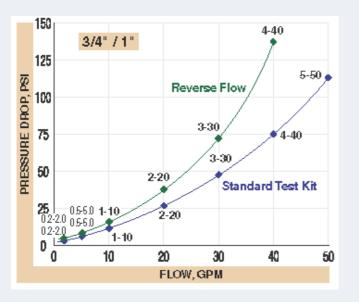
Graph 1: p/Q characteristic curve for pressure drop (blue) for a standard <sup>3</sup>/<sub>4</sub>" and 1" power meter
