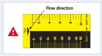
1. Mount the volume flow meter so that the fluid flows in the direction of the flow arrow.
